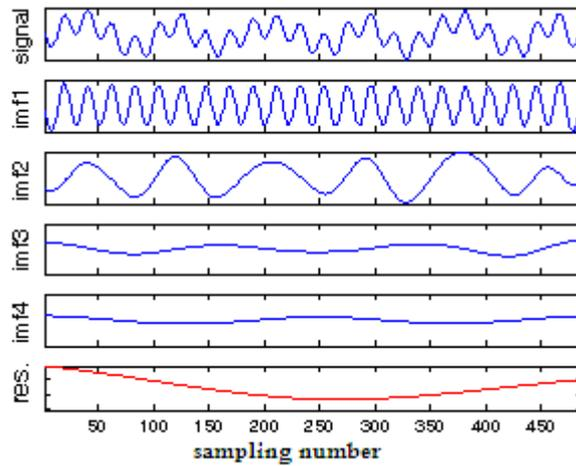
Fig. 10. EMD Decomposition before End Extending
