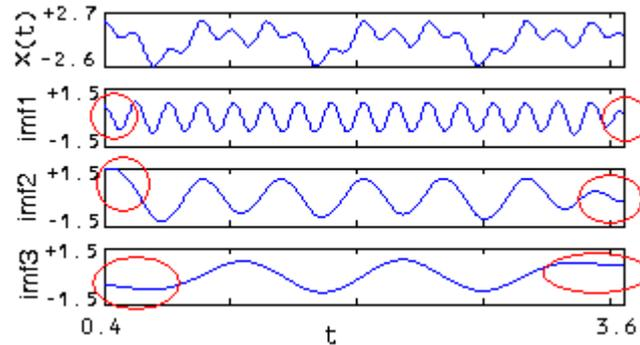
Fig. 2. Result of EMD Decomposition
