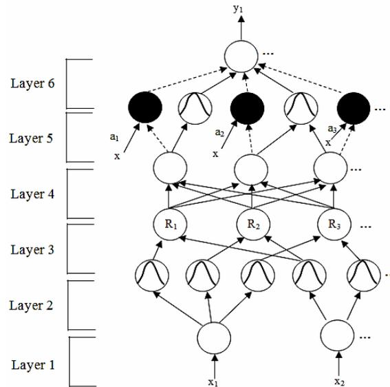
Fig 1. The structure of SONFIN
