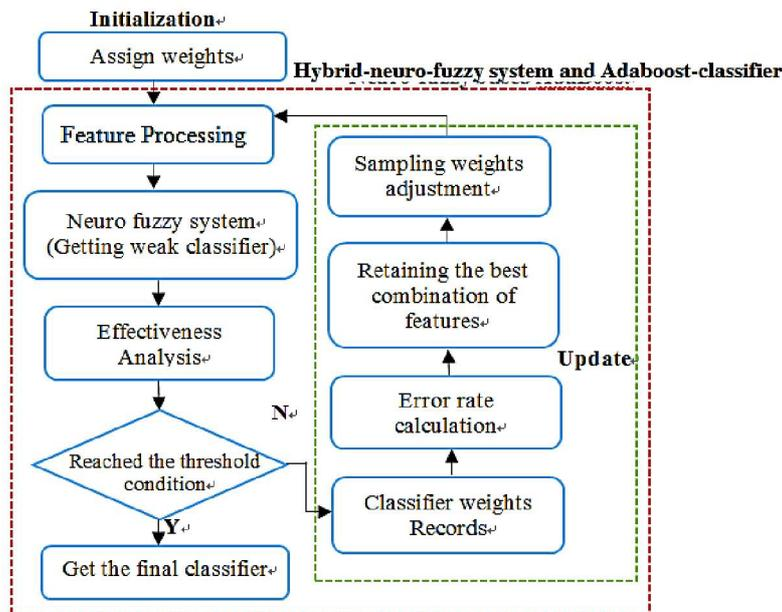
Fig. 2. The architecture of Hybrid-neuro-fuzzy system and Adaboost-classifier classifier
