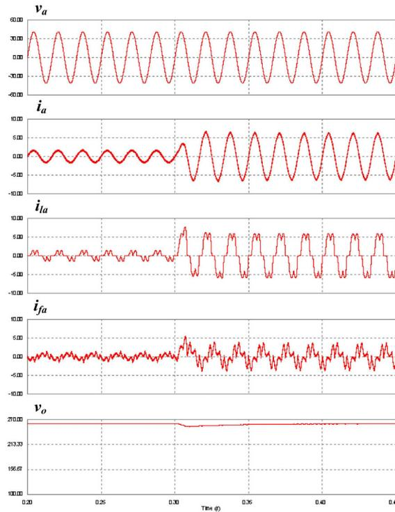
**Fig. 7.** A-phase phase-to-neutral voltage  $v_a$ , line current  $i_a$ , the load current  $i_{la}$ , the compensation current  $i_{fa}$ , and the dc capacitor voltage  $v_o$  under a step load change from 60 W to 310 W
