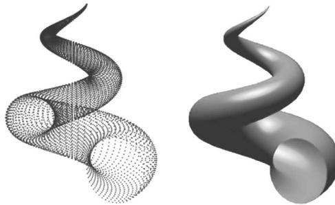
**Fig. 2.** Shell point cloud (left) and fitting surface (right)
