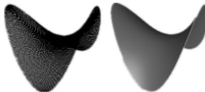
**Fig. 1.** B-spline point cloud (left) and fitting surface (right)
