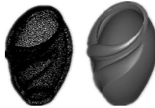
**Fig. 4.** Vase point cloud (left) and fitting surface (right)
