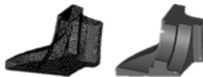
**Fig. 6.** Fandisk point cloud (left) and fitting surface (right)
