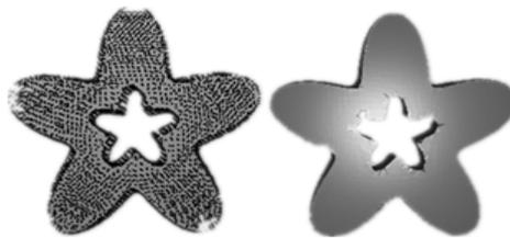
**Fig. 5.** Trim-star point cloud (left) and fitting surface (right)
