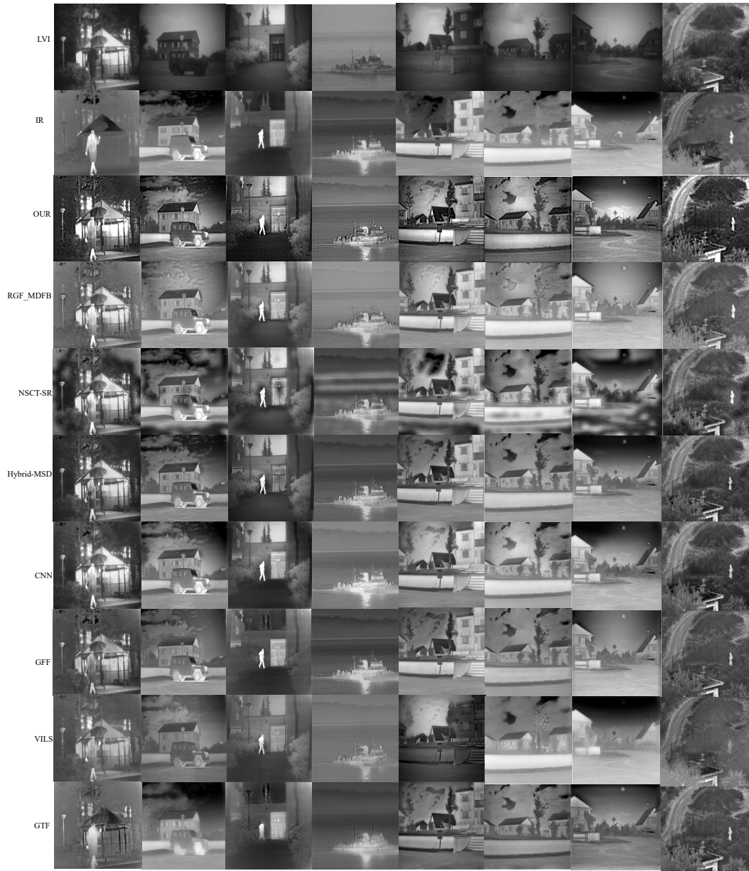
Fig. 4. The infrared and low illumination visual image and the infrared and visual image fusion of the different fusion algorithms
